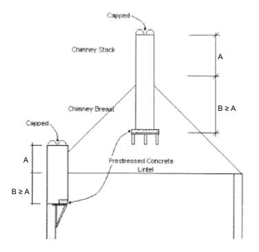
Note: B must be equal to or greater then A Above; Minimum height of the chimney breast remaining in the house is the height of brickwork in the stack above.
