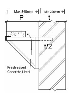
Above; Chimney Breast cannot exceed 340mm The minimum thickness of the wall is 225mm
